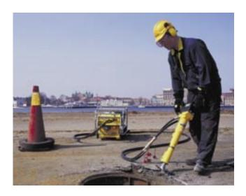
Hydraulics are reliable by nature. Working in a closed loop, dirt and moisture are kept out. And due to the no-spill, flat-face couplings, it's easy to keep the system clean.
